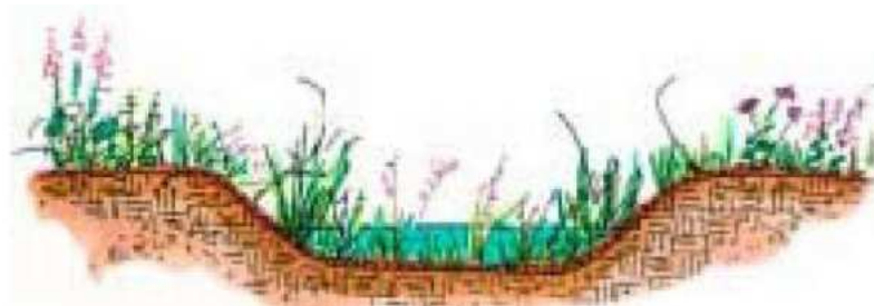
Figure 10.4.2 Naturalized Infiltration Basin (Improving Stormwater Basin Design, 2008)
