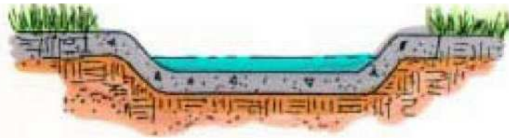
Figure 10.4.1 Traditional Infiltration Basin (Improving Stormwater Basin Design, 2008)
